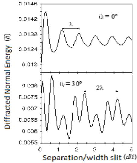
**Figure 4.** Energy diffracted in the direction normal to the standard  $E_i$  to Hermite-Gauss beam, depending on the spacing  $d/l$  screen. For the fundamental mode  $m = 0$ , at normal incidence and oblique incidence of  $30^\circ$ , with  $\lambda/l=0.9$ ,  $L/l=500/\sqrt{2}$ ,  $h/l=1$ ,  $y b/l=0.5$ .
