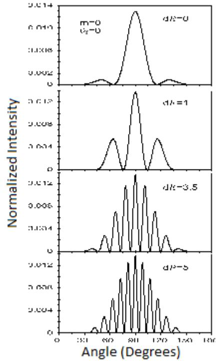
**Figure 2.** Diffraction patterns normalized  $(I(\theta)/I_0)$  of Hermite-Gaussian beams of  $m = 0$  normally incident on two slits so. With  $\lambda/\ell = 0.9$ ,  $L/\ell=500/\sqrt{2}$ ,  $h/\ell = 1$  and position  $b/\ell=0.5$  and for separations  $d/\ell = 0, 1, 3.5$  and  $5$ .
