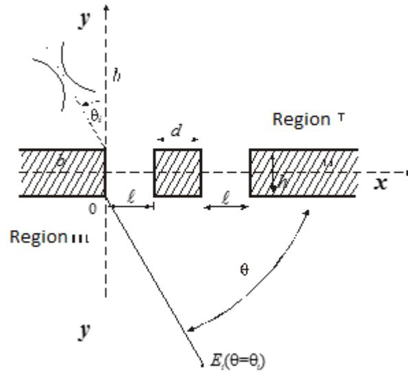
**Figure 1.** Our system. Two slits of width  $\ell$  and spacing  $d$  in an infinitely thick conducting screen  $h$ . The energy diffracted along the incident direction ( $E_i$ ) is diffracted in the direction of  $\theta$  (relative to the axis  $Oy$ ) =  $\theta_i$  (From the axis  $Ox$ ).
