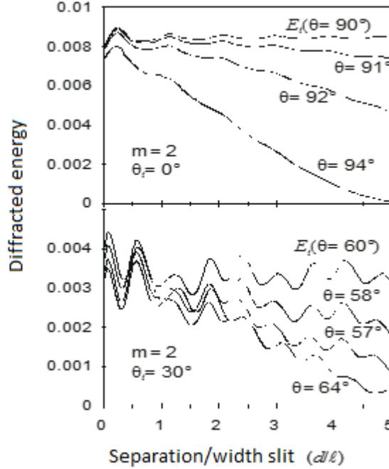
**Figure 6.** Energy diffracted around energy  $E_i(\theta = \theta_i)$  Hermite-Gauss beam, for the  $m = 2$  mode according to the distance between slits  $d/\ell$ . Same parameters of Fig. 4.
