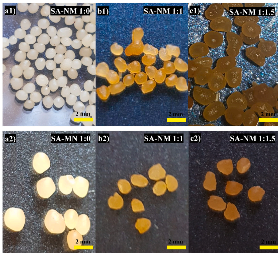
Fig. 1. Optical microscopy images of external surface and shape of the hydrogel beads and dry beads for (a) SA-NM (1:0); (b) SA-NM (1:1) and (c) SA-NM (1:1.5).
