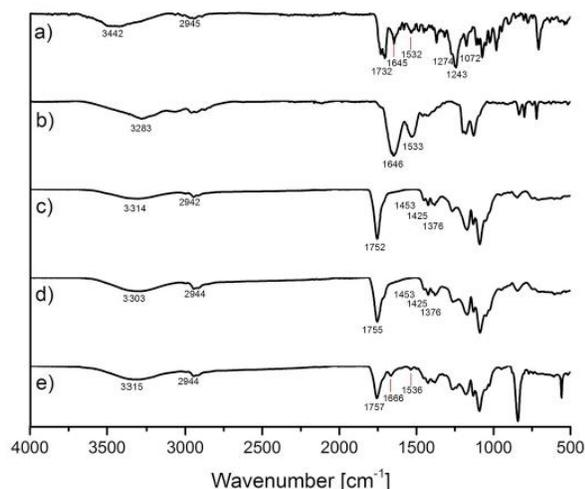
Fig. 3. Infrared spectra of a) paclitaxel, b)  $\text{Lys}^1\text{Lys}^3(\text{DOTA})\text{Bombesin}$ , c) PLGA nanoparticles d) PLGA(PTX) nanoparticles and e) BN-PLGA(PTX) nanoparticles.
