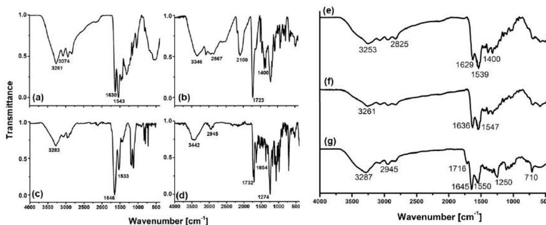
**Figure 3.** The FT-IR spectrum of (a) PAMAM Dendrimer (DN), (b) pSCN-Bn-DOTA (DOTA), (c)  $\text{Lys}^1\text{Lys}^3(\text{DOTA})\text{-BN}$  (BN), (d) Paclitaxel (PTX), (e) DOTA-DN, (f) DOTA-DN-BN, (g) DOTA-DN(PTX)-BN.
