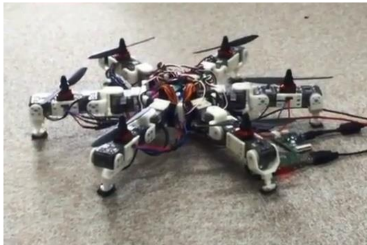
Figure 8. Hybrid robot for bridges inspection [30]
