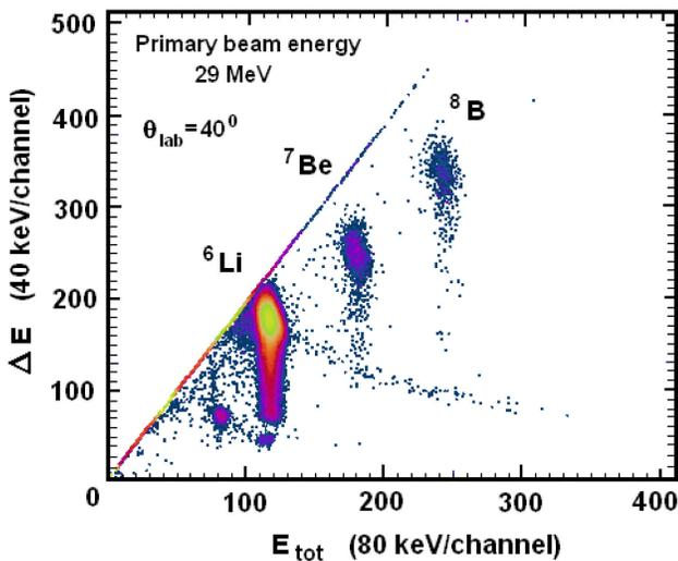
FIGURE 1. Two-dimensional spectrum obtained with  $E-\Delta E$  telescope. The elastic scattering groups for  ${}^8\text{B}$ ,  ${}^7\text{Be}$ , and  ${}^6\text{Li}$  are indicated.
