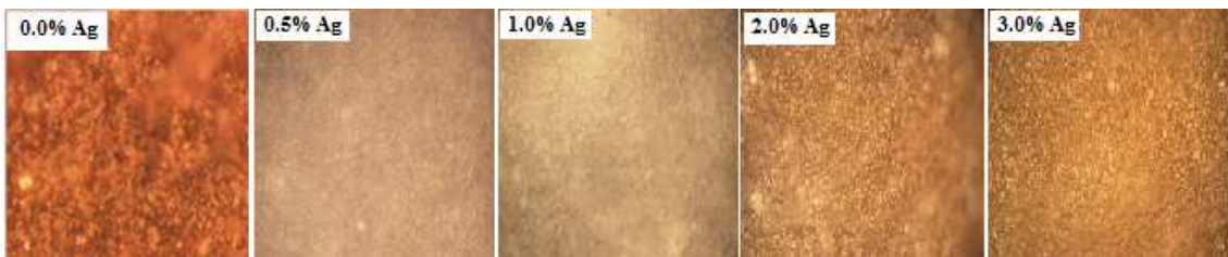
Figure 5. Optical micrographs of Al 2 O 3 /Ag samples sintered at 1500 °C during 2 h.
