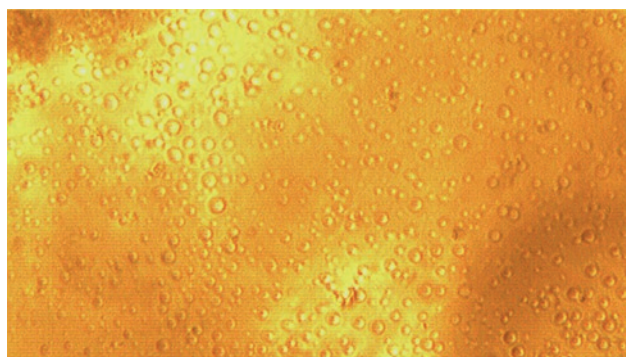
Figure 8: Digital image of methanol drops in an oil continuum, methanol-oil molar ratio = 6.
