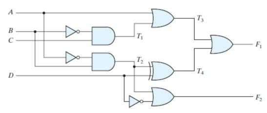
$$F_1 = T_3 + T_4 = A + B'C + (A'BD' + (A + B')D) = A + B'C + A'BD' + AD + B'D$$
