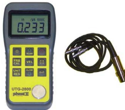
Figura 24. Ultrasonic Thicknees Gauge (Phase II) modelo
