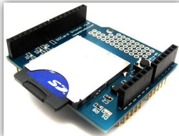
Figura 14 Shield SD Arduino
