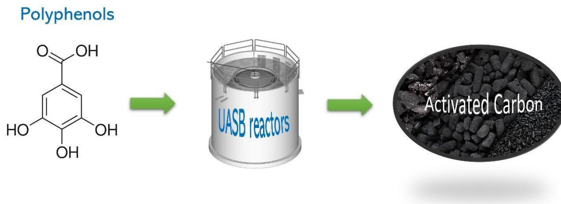
Fig. 12. PPs removal using activated carbon after biochemical treatment Upflow Anaerobic Sludge Blanket (UASB) Reactors (own creation).
