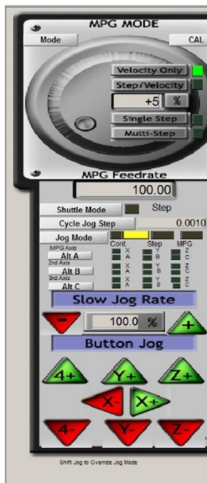
Illustration 10. Mach 3 manual control interface, it appears after pressing "tab".
