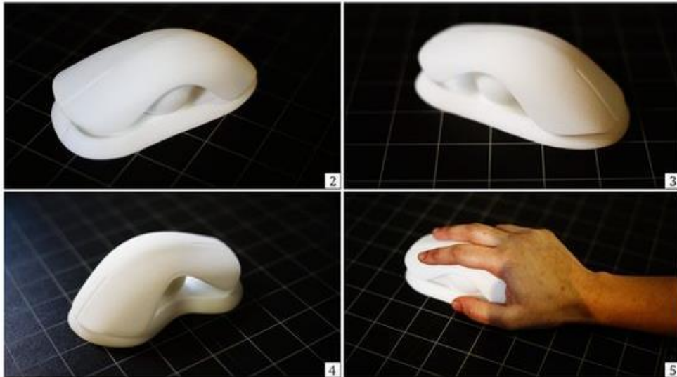
1-5. Rapid Prototype Model, created to assess the movement and functionality of the sphere mechanism. The Model was created from CAD data and 3D printed on a SLS Rapid Prototype Machine
