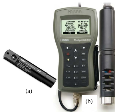
Figure 3. Equipment used: (a) HOBO Conductivity Logger U24-001 and (b) HI 9828.
