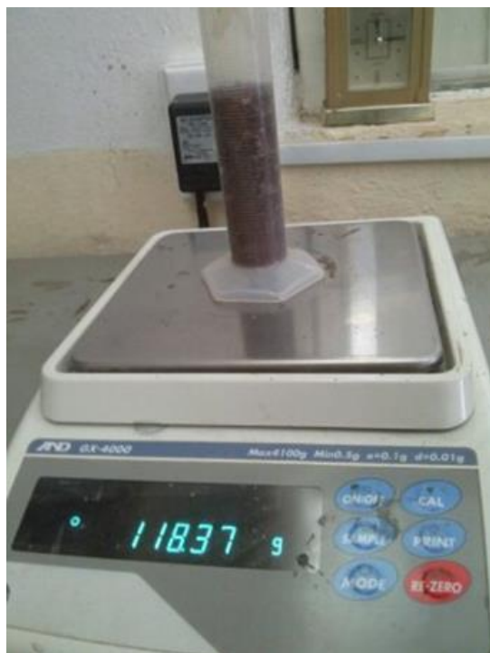
Figure 4 Weight of water and natural porous material in the volume occupied by the material
